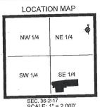
BASIS OF BEARING: ALL BEARINGS REFER TO GRID NORTH OF THE WISCONSIN STATE PLANE COORDINATE SYSTEM, SOUTH ZONE. THE SOUTH LINE OF THE SE 4 OF SEC. 31-2-19 WAS ASSUMED TO BEAR N88°11'55"W
