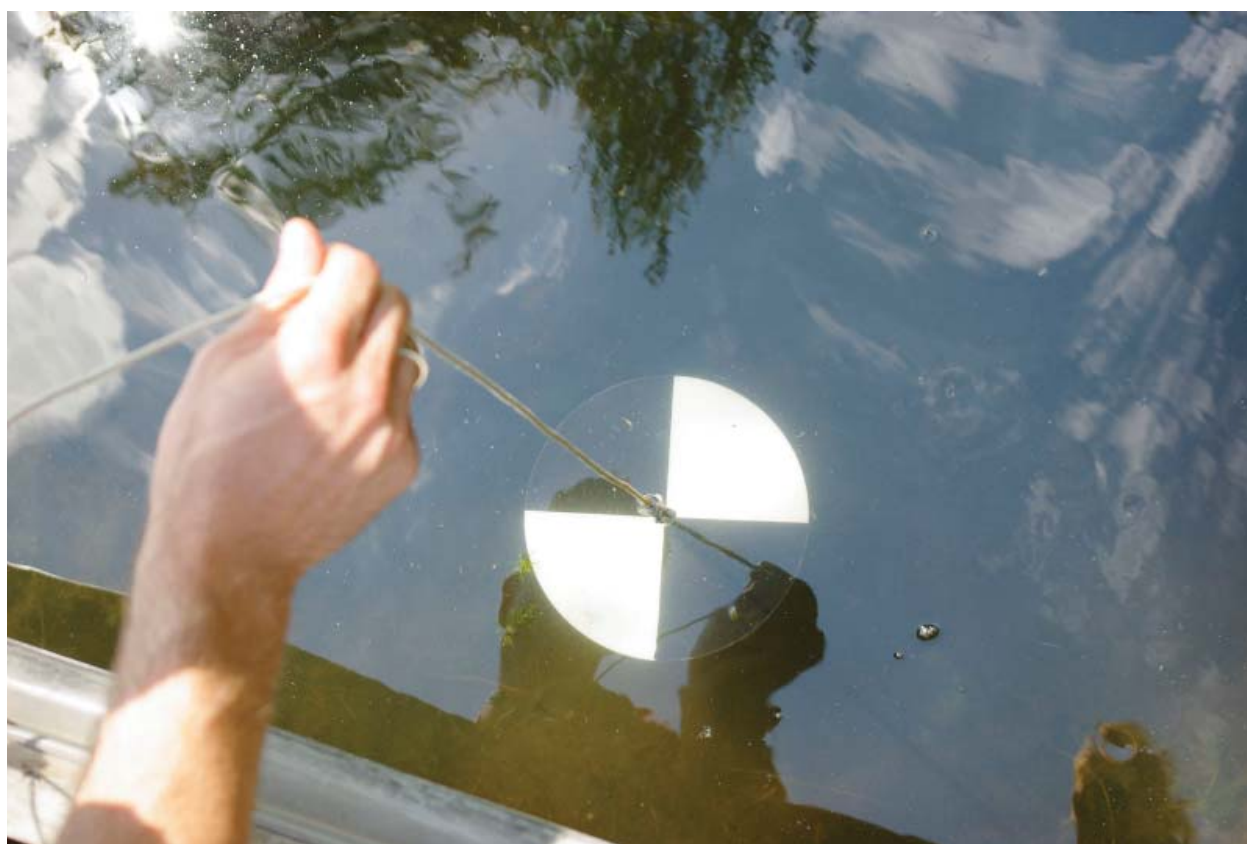
Figure 3 Measuring Water Clarity with a Secchi Disk
