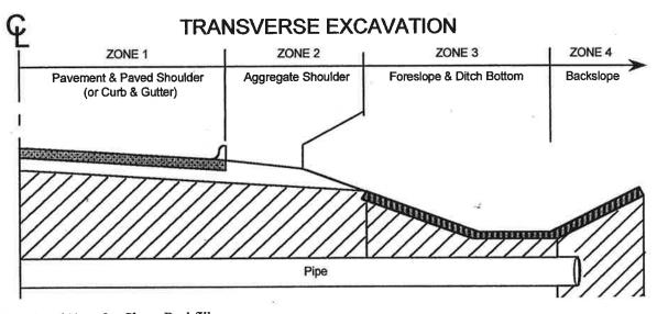
Zone 1 and Zone 2 - Slurry Backfill
