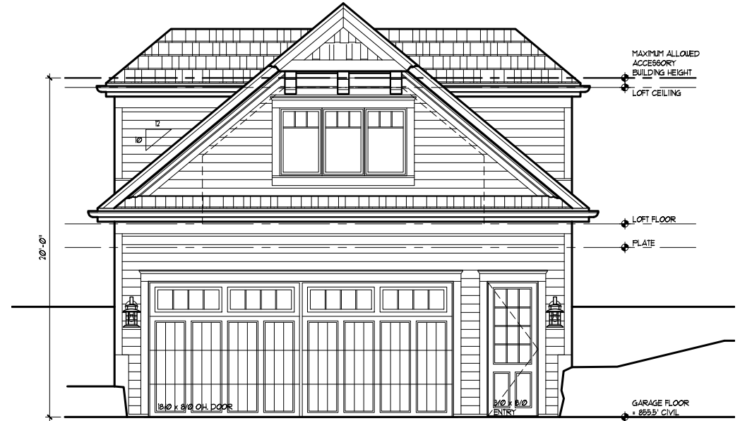
NORTHWEST (STREET) ELEVATION SCALE: 1/8" = 1'-0"
