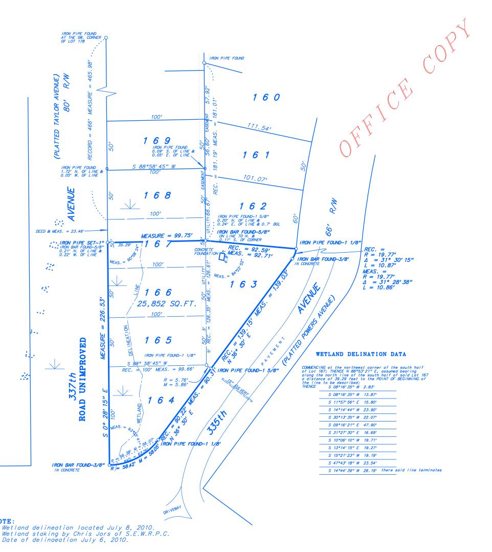
A Jeffery K. Rampart survey for a Lot Line Adjustment involving Lot 167 and Lot 168, dated June 24, 2002, indicates iron pipes set at the corners for the division of Lot 167, which no pipes were found. Also Statute A—E7.05(4)was not followed for the establishment of the corners set on a stable across reference at the corner set of let 168 the corner reference at the northwest corner of Lot 168.
