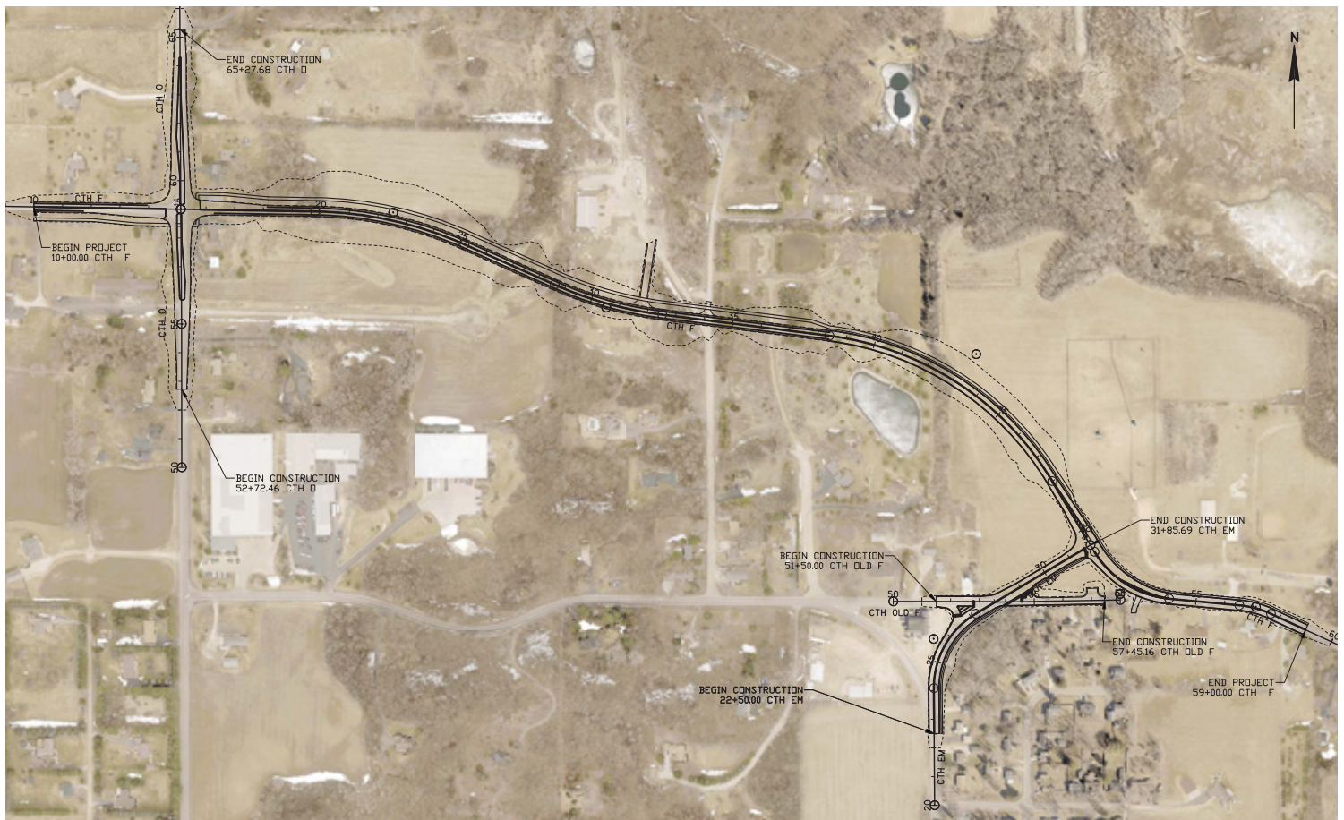
30% Preliminary Design layout for CTH F extension
