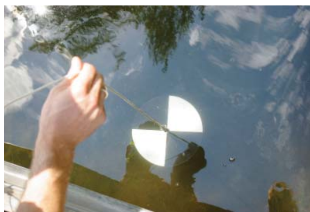
Figure 5 Measuring Water Clarity with a Secchi Disk
