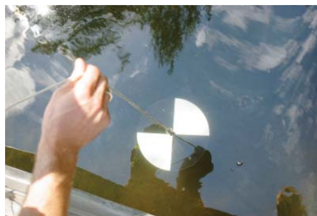
Figure 4 Measuring Water Clarity with a Secchi Disk
