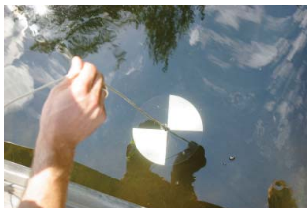
Figure 3 Measuring Water Clarity with a Secchi Disk
