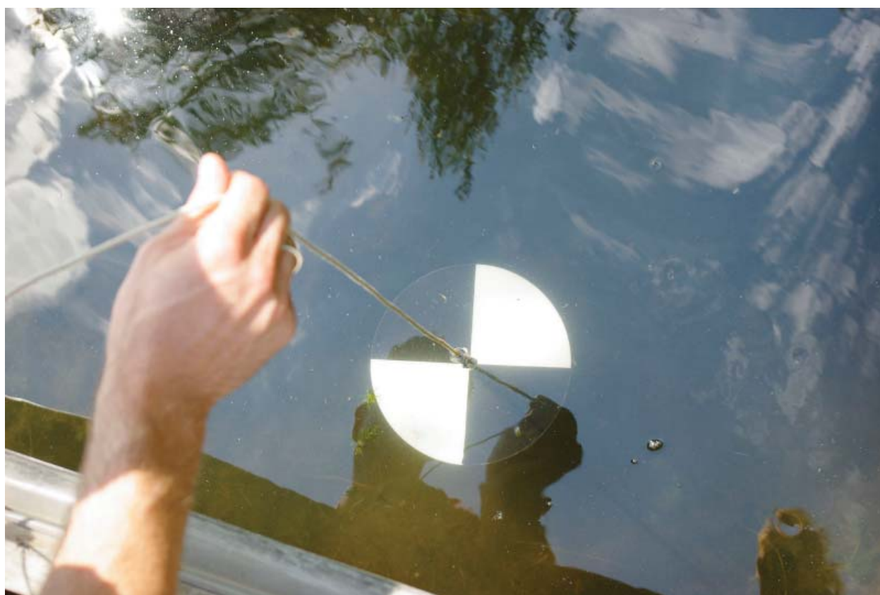
Figure 3 Measuring Water Clarity with a Secchi Disk
