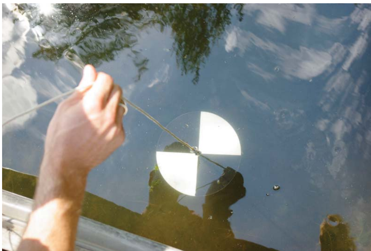
Figure 4 Measuring Water Clarity with a Secchi Disk
