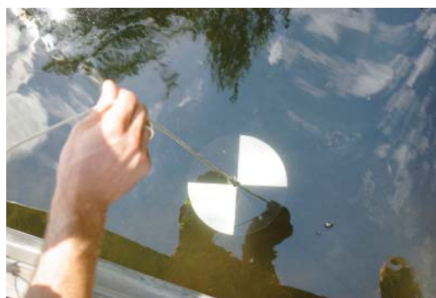
Figure 4 Measuring Water Clarity with a Secchi Disk
