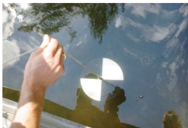
Figure 3 Measuring Water Clarity with a Secchi Disk
